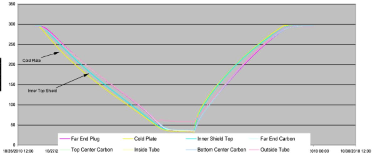
Figure 12. Temperature profiles during thermal cycle of ISIM tube in CDMF chamber
