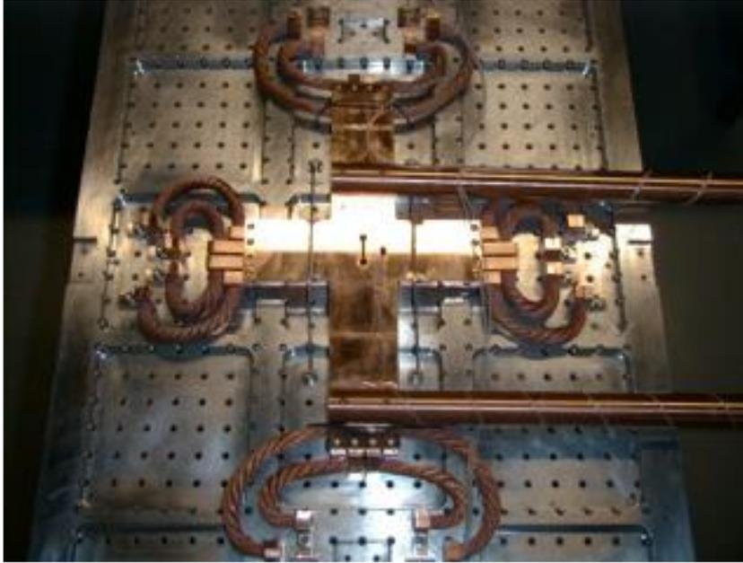
Figure 4 Connection of thermal bus to cold plate
