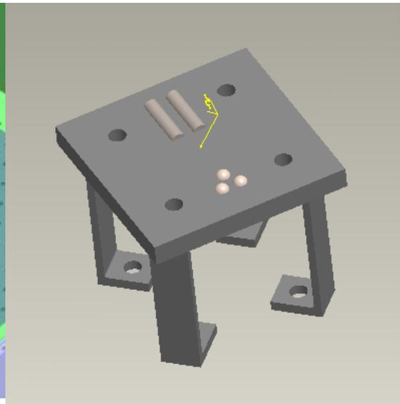
Figure 8 Kinematic positioning
