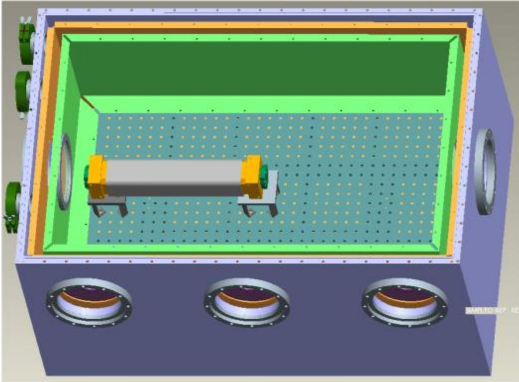
Figure 2. Isometric view of the CDMF cryochamber, showing a tube placed on the cold plate.
