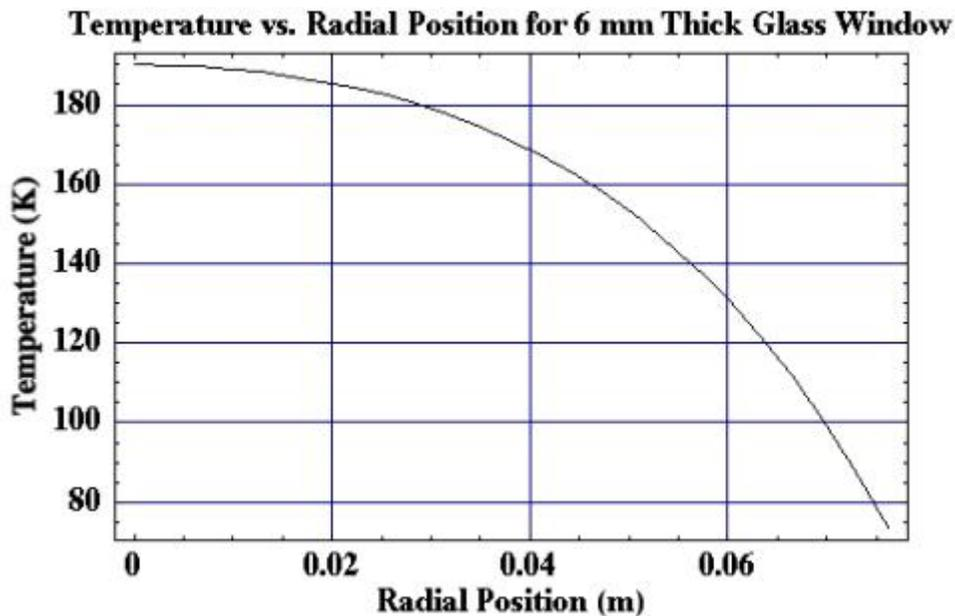
Figure 5. Modeled temperature of glass radiation shield on outer thermal shroud
