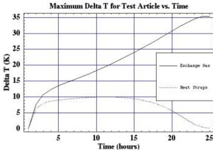
Figure 6. Thermal gradient in test part in modeled cooldown.
