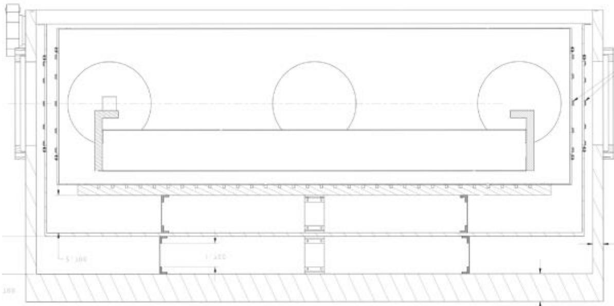
Figure 3. Side view of the cryo-chamber, showing the thick vacuum walls, the two thermal shrouds set off by insulating flexures, the cold plate with attached test article, and in the back walls, three metrology ports.
