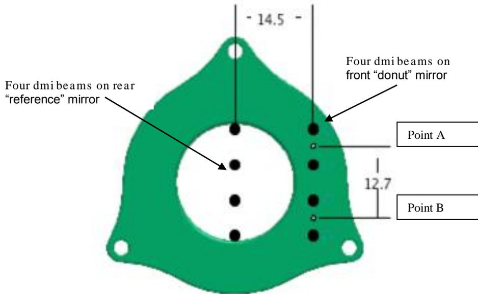
Figure 11 Beam locations of the two compact interferometers
