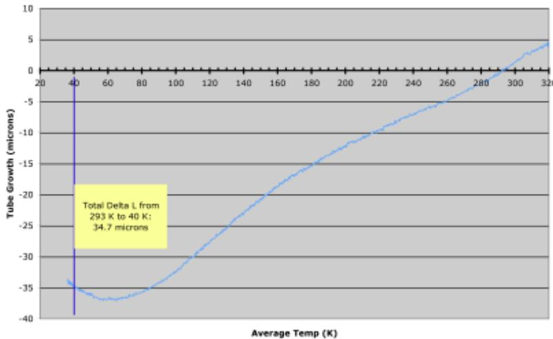
Figure 14 Sample run of CDMF: Delta L vs. temperature
