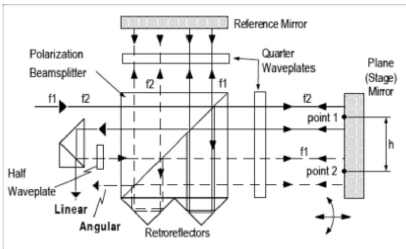
Figure 10 Diagram of compact interferometer
